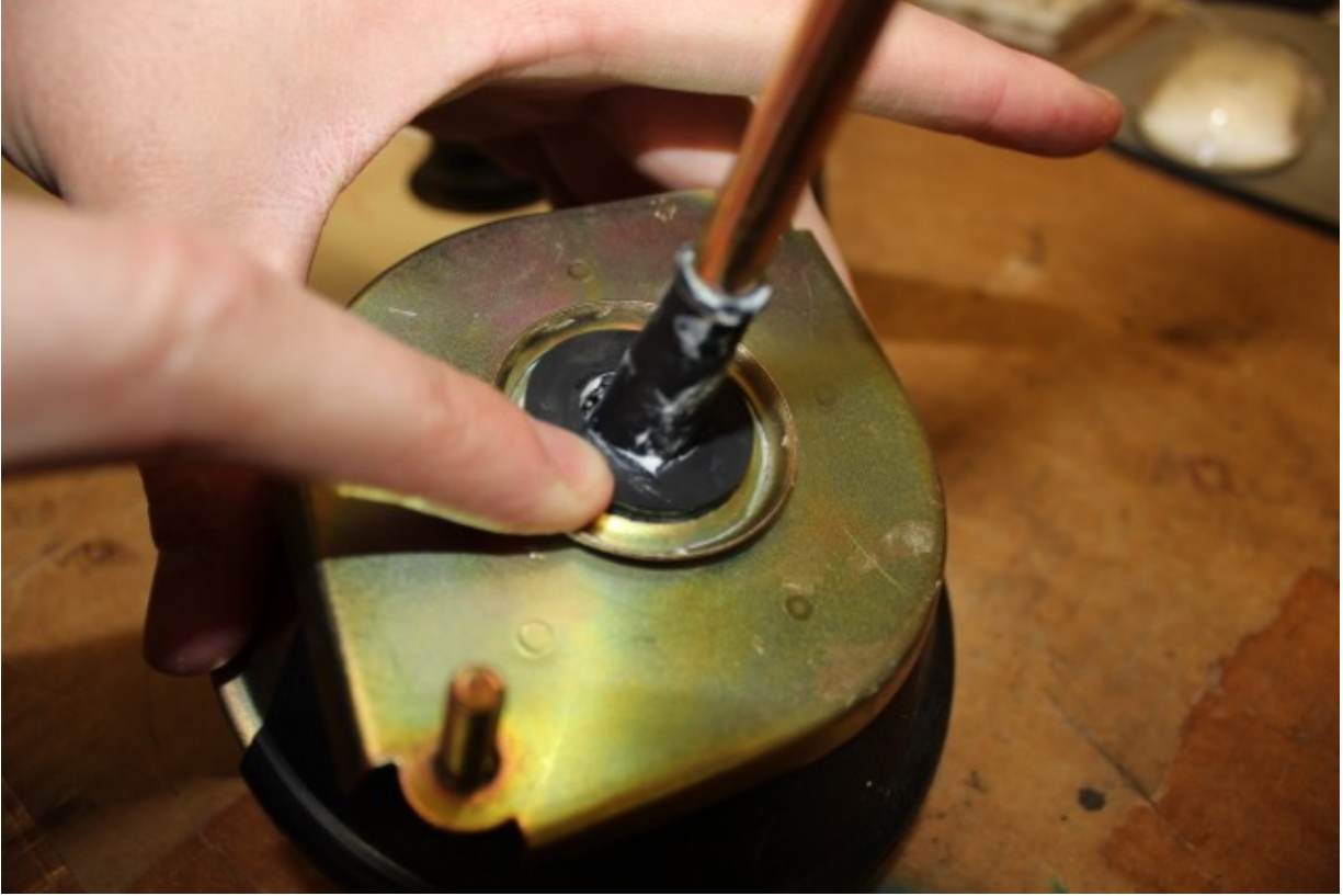
Using the same grease, coat the friction area of the outer boot on the inside.
