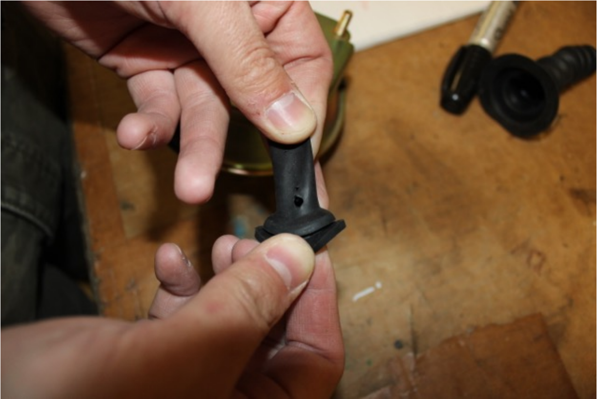
Using a grease like a white lithium grease, apply to the friction area of the inner seal.
